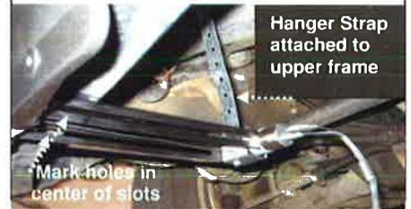
D. Alternatively, if there is a lip air dam and a mounting spacer is required, cut two lengths from the steel strip and bend each in a "Z" shape per the photo below. Use screws and nuts provided.
